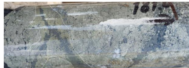
Sphalerite veinlet (Zinc sulphide - dark area) with chalcopyrite margin in massive sulphide interval
